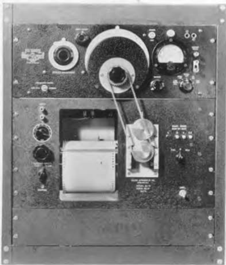
Figure 1. View of the Sound Apparatus Company's Model SL-4 Recorder coupled to the General Radio Type 1304-B Beat Frequency Audio Generator.
