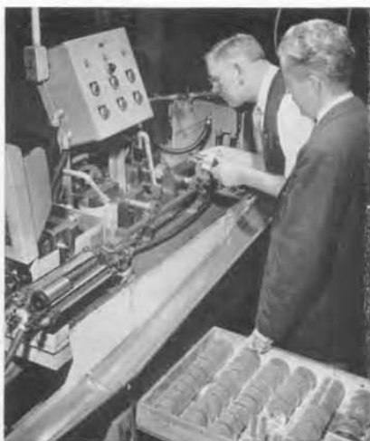
Figure 3. Designed and built in General Radio's tool department, this machine automatically mills the rotors and stators from the aluminum extrusions shown in Figure 4.
